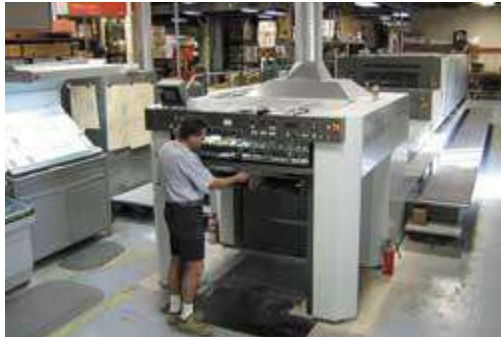
Pressman Matt McGrath beginning a make ready on the Komori LS 6-color with coater.
